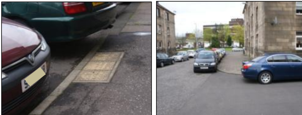
Figure 2.7 – Pedestrian Facility Blocked by On-Street Parking and Parking at Junctions
